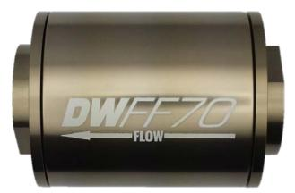
DW fuel filters are compatible with a wide range of fuels including pump gas, race gas, MTBE, ethanol, methanol, and diesel. DW reccommends a maximum service interval of 12 months or 12,000 miles. Shorter service intervals are reccomended with harsher conditions and corrosive fuels.
